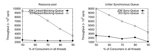
Fig. 6. Performance changes of a Resource pool and unfair SynchronousQueue when total number of threads is 64, as the ratio of consumer threads grows from 50% to 90% of total thread amount.
