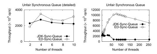
Fig. 3. The unfair synchronous queue benchmark: a comparison of the latest JDK 6.0 algorithm and our novel ED-Tree based implementation. The graph on the left is a zoom in of the low concurrency part of the one on the right. Number of producers and consumers is equal in each of the tested workloads.
