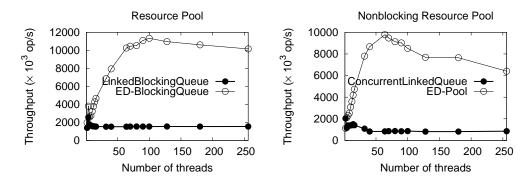
Fig. 4. Throughput of BlockingQueue and ConcurrentQueue object pool implementations. Number of producers and consumers is equal in each of the tested workloads.
