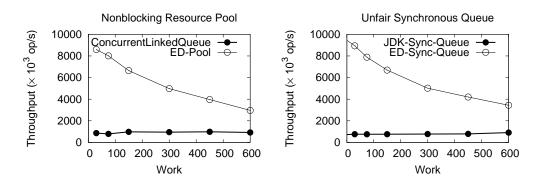
Fig. 5. Throughput of a SynchronousQueue as the work load changes for 32 producer and 32 consumer threads.)
